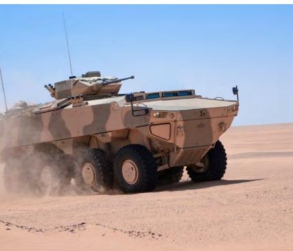
The PARS III 8x8 vehicle runs ahead of its competitors by offering ballistic and mine protection levels similar to MRAP vehicles while maintaining combat and mobility characteristics of modern armoured combat vehicles. The PARS III 8x8 has an integrated air-conditioning system, which keeps the vehicle's internal temperature at +25 °C even in the hottest desert conditions.
