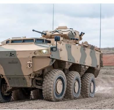
The hull form, underbelly structure, base plates and specially developed mine-resistant seats are designed to protect personnel against high-level mine threats. The PARS III 6x6 vehicle runs ahead of its competitors by offering ballistic and mine protections levels similar to MRAP vehicles while maintaining combat and mobility characteristics of modern armoured combat vehicles.
