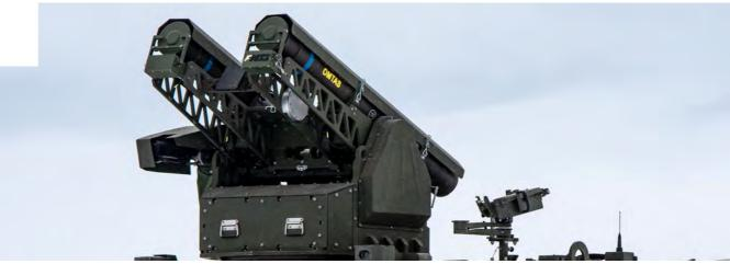
The ARCT was designed specifically for the anti-tank role from the very outset and has some important integrated features that turrets with add-on missile capability are lacking. The ARCT offers the best optimization for low silhouette, armour protection, ergonomics, easy conversion to tripod launch configuration and sighting system.
