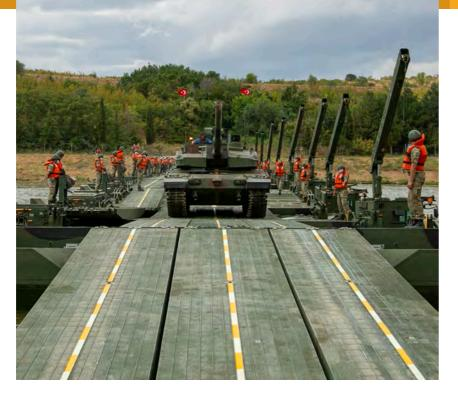
In terms of self-sufficiency, the OTTER can carry four ramps on a single system, which eliminates the need for additional logistic vehicles. The OTTER is also fitted with a self-recovery winch, which recovers the vehicle or any other system especially in soft terrains.
