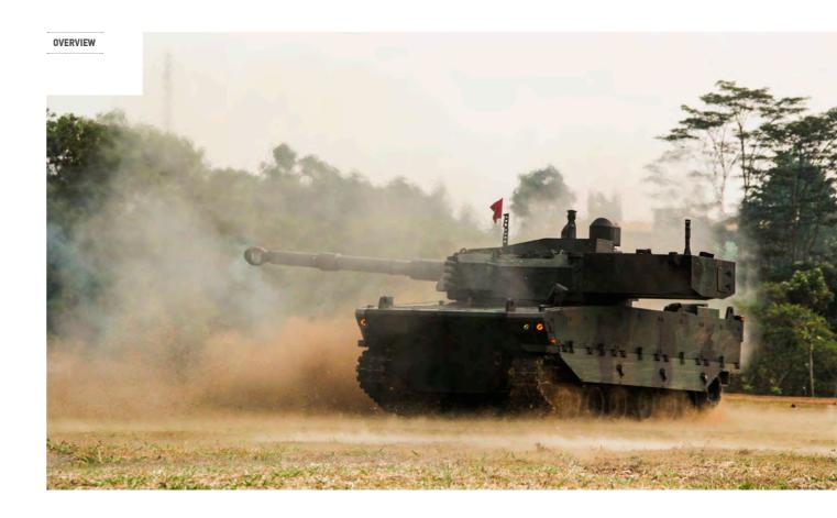
The new generation KAPLAN MT is the sole and exclusive modern Medium Weight Tank designed with rear powerpack and not a conversion of a variant from an existing IFV.
