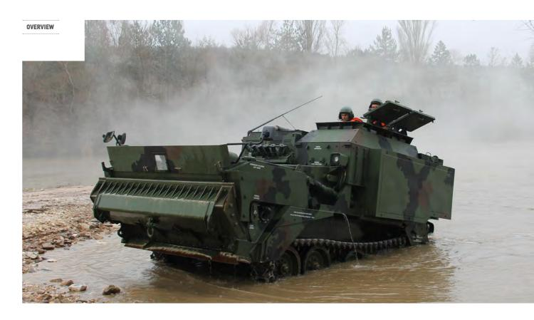
The AACE is an amphibious, armoured, tracked, combat earthmover, designed for the preparation of river banks during river crossing missions. It is capable of performing bulldozing, rough grading, excavating, hauling, and scraping operations.
