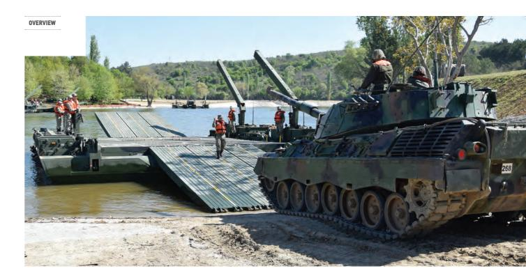
The OTTER is a bridge and ferry system designed for safe and fast transport of combat and logistic military vehicles in river crossing operations.
