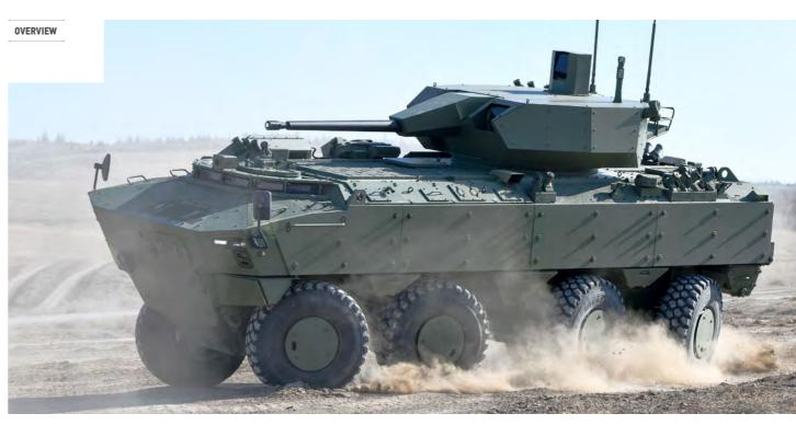
The PARS IV 8x8 New Generation Wheeled Armoured Vehicle (NG-WAV) was designed and produced with FNSS' equity, considering the technical features that have evolved according to future requirements and the demands from armies worldwide. The vehicle combines user ergonomics with protection and high mobility.
