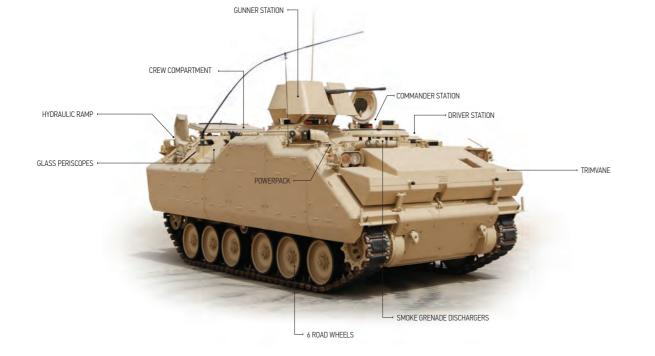
The vehicle is upgradeable thanks to its growth potential and its configuration can be tailored in accordance with user requirements into a true family of vehicles that can be utilized as cavalry, infantry, MBT's support vehicles and artillery.
