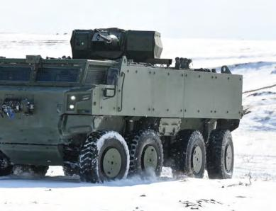
The PARS SCOUT 8x8 hull can be brought to the level of protection required thanks to its modular-designed armour system. The hull shape, underbelly structure, bottom plates and specially developed mine-resistant seats are designed to protect personnel against high-level mine threats.
