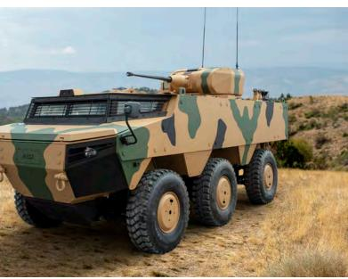
The PARS SCOUT 6x6 hull can be brought to the level of protection required thanks to its modular-designed armour system. The hull shape, underbelly structure, bottom plates and specially developed mine-resistant seats are designed to protect personnel against high-level mine threats.
