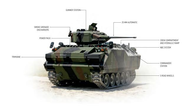
The all-welded construction provides a watertight hull; and hatches, doors, and other openings have watertight seals. The power plant and the driver's and commander's compartments in the forward area utilize about half the space, the turret section, and the personnel compartment in the rear utilizes the remaining half.
